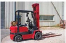
Forklift trucks that run on propane are alternatives to those that run on gasoline or diesel fuel.
