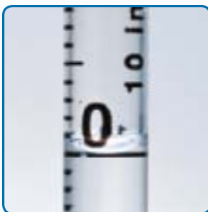
Figure D Always read the volume of the solution at the bottom of the meniscus.
