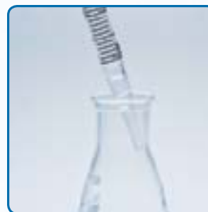
Figure E Draining the pipette with the tip against the wall of the flask will prevent splashing.
