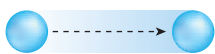
Figure 11.4 This model of a particle depicts translational motion—the motion of something that moves freely from one place to another.
