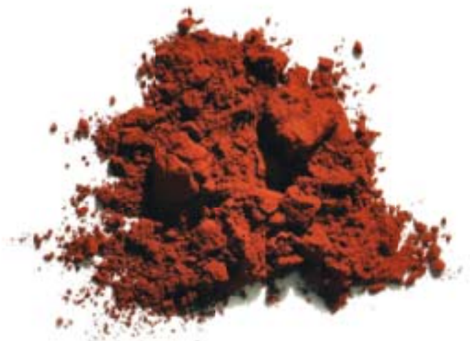
Figure 3.3 Iron(III) oxide is an inorganic solid with the formula \text{Fe}_2\text{O}_3 . In nature, this substance is the mineral hematite, which is a principal source of iron for the mining industry. Since prehistoric times, people around the world have used iron(III) oxide as a colouring agent (pigment) for painting. In this context, the substance is often called red ochre.
