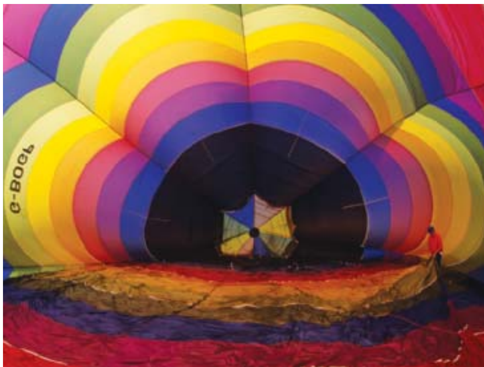
Figure 3.11 This hot-air balloon is made from a flame-resistant fabric. The same type of fabric is also used for such applications as making protective clothing for firefighters.
