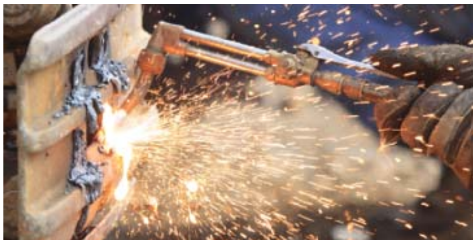
Figure 3.22 This welding torch uses acetylene, a hydrocarbon, as fuel.
