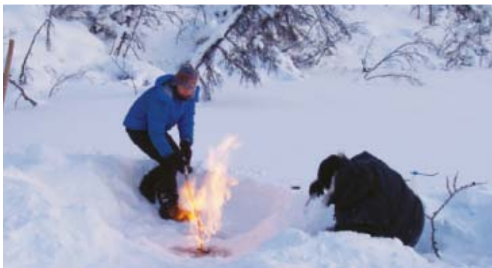
Figure 3.20 University of Alaska Fairbanks researcher Katey Walter lights a pocket of methane on a thermokarst lake in Siberia in March of 2007. Igniting the gas is a way to demonstrate, in the field, that it contains methane.
