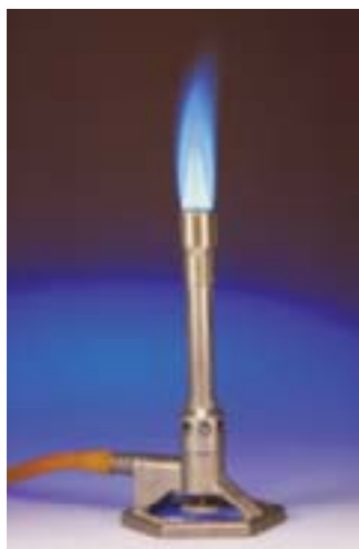
Figure 3.23 A blue flame indicates that complete combustion is occurring.
