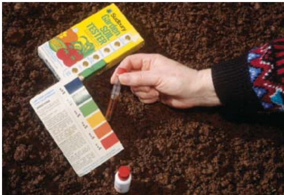
Figure 4.11 Depending on the results of this soil test, lime, \text{CaO}(s) , might be added to neutralize excess acids in the soil, or a substance such as ammonium sulfate might be added to neutralize bases.
