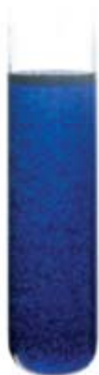
Figure 4.19 The precipitate that is formed in the reaction between sodium iron(II) cyanide and iron(III) chloride is a pigment known as Prussian blue. This pigment is used in blueprints and paints.
