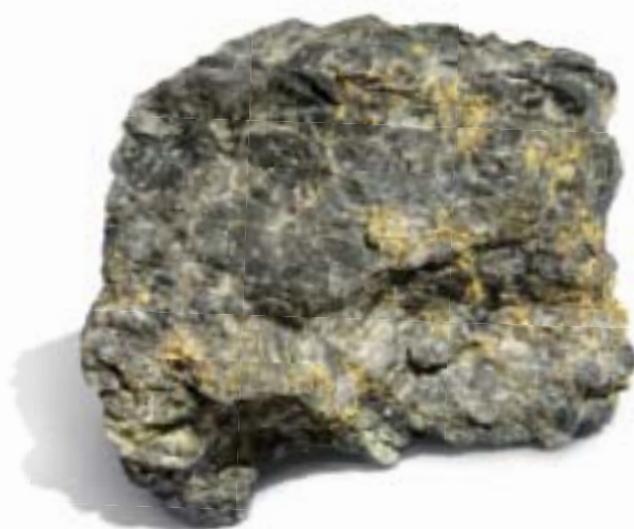
Figure 4.18 Much of the rock mined as gold ore contains particles of gold that are too tiny to be seen without a microscope. Some rocks, however, such as the one shown here, contain visible particles of gold.
