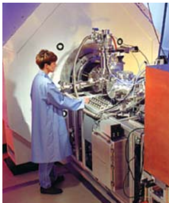
Figure 5.7 This elaborate device is called a mass spectrometer. It is used to make precise mass measurements and to determine molecular structure.
