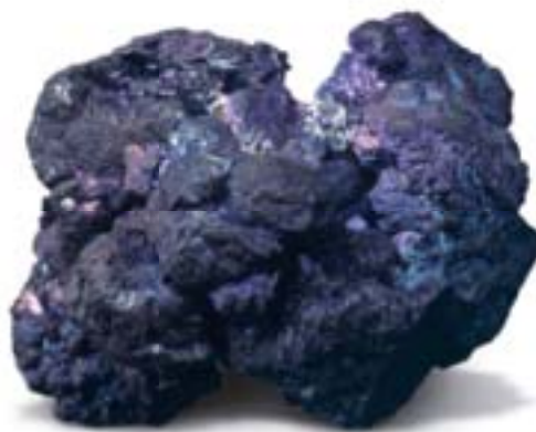
Figure 6.5 Chalcocite is a copper ore. Most metals are found in impure rocks and mineral ores, which must be refined to obtain the pure metals. Knowledge of percentage composition is necessary for metallurgists who want to assess the values of ores and mineral deposits.
