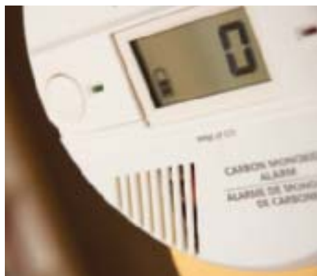
Figure 7.9 Propane can produce carbon monoxide during incomplete combustion. Because carbon monoxide is poisonous, detectors are used in homes to warn people if the gas is present.
