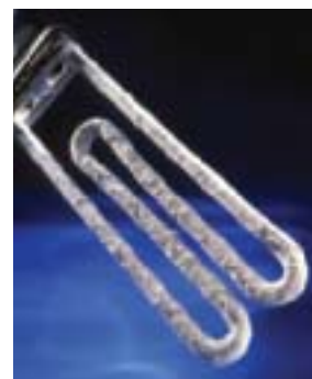
Figure 9.17 Deposits of calcium carbonate and magnesium carbonate on water-heating elements can reduce the heater's efficiency.
