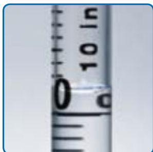
Figure C Start with more of the unknown solution than you need. You will drain out the excess solution in the next two steps.
