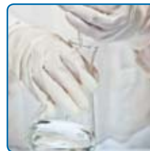
Figure J Always swirl the flask as you add the titrant. If you have trouble swirling and adding titrant at the same time, use a magnetic stirrer or have your laboratory partner swirl the flask as you add the titrant.
