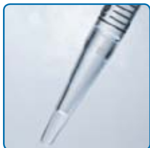
Figure F A small amount of solution will always remain in the tip of the pipette. Do not remove this.
