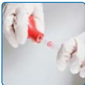
Figure A Squeeze the pipette bulb as you put it on the stem of the pipette.
