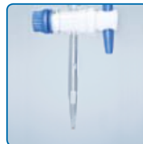
Figure H Do NOT start a titration if you have air bubbles like these in the tip of the burette. They will cause errors in your measurements.
