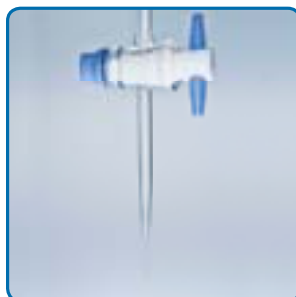
Figure G The tap is fully open when the handle on the tap is parallel to the burette and the solution inside the burette comes out quickly.
