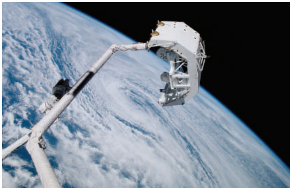
Figure 11 Weighing 450 kg, the Canadarm can pick up and move objects that weigh as much as 29 tonnes. Astronauts use computers within the space shuttle to control this robotic crane.
