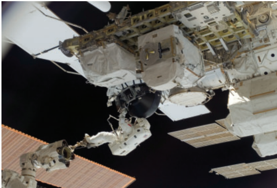
Figure 12 Anchored to the foot restraint on the Canadarm, Canadian astronaut Dave Williams spent 6.5 hours replacing a faulty piece of equipment on the ISS.
