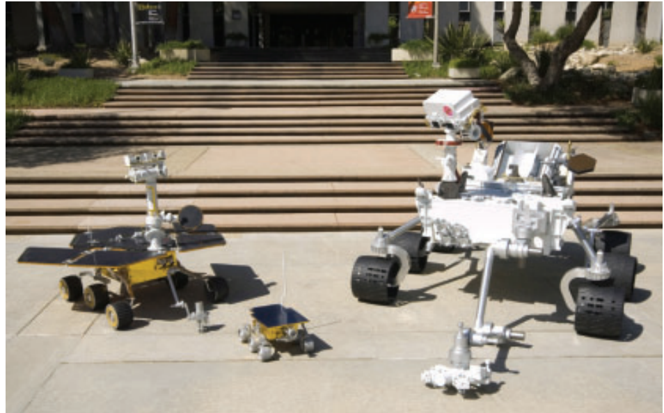
Figure 3 Three generations of Mars rovers: the two on the left used solar panels to generate power; the new, larger Mars rover uses a nuclear generator, giving it many times more power.
