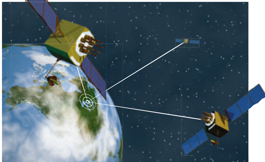
Figure 4 A GPS receiver's position on Earth can be accurately determined by using triangulation, which is the measure of the distance between the receiver and three orbiting GPS satellites.
