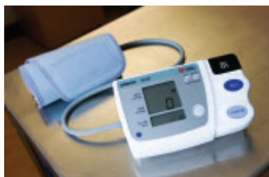
Figure 7 The portable device used to monitor blood pressure is called a sphygmomanometer.
