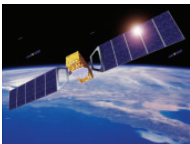
Figure 3 The wing-like solar panels of a GPS satellite absorb radiation from the Sun, which is then stored in batteries.
