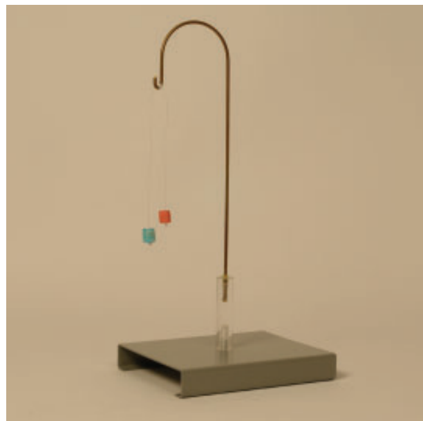
Figure 2 A double pith ball electroscope consists of two neutral pith balls hanging side by side.
