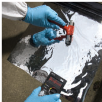
Figure 4 An electrostatic lifting apparatus is used in forensics to create a copy of a footprint from a crime scene.
