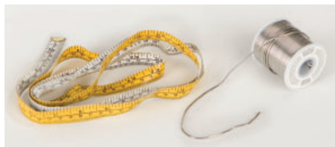
Figure 7 Solder is used to form solid connections between wires and copper pipes. You will be measuring the ductility of solder.
