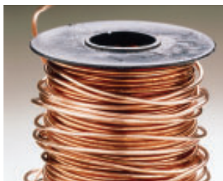
Figure 12 Copper wire is considered ductile.
