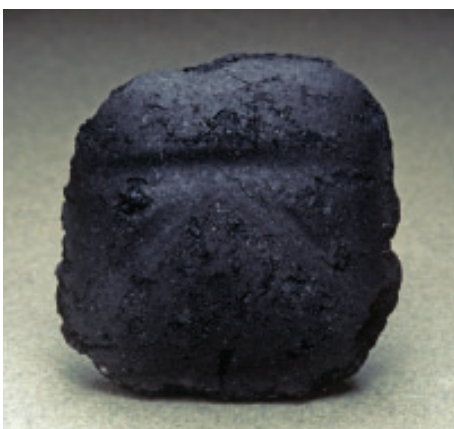
Figure 8 A charcoal briquette is made up of 85 % to 98 % carbon. Carbon, a non-metal, is dull and brittle.
