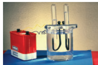
Figure 2 When an electric current passes through water, the particles of water are split apart, producing two gases—hydrogen and oxygen.
