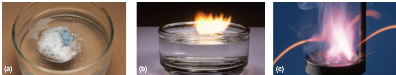
Figure 1 Lithium (a), sodium (b), and potassium (c) react at different rates with water to produce flammable hydrogen gas. The reactions release so much thermal energy that the hydrogen gas ignites.
