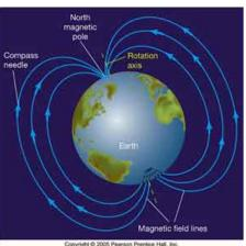
If you are navigating using a magnetic compass, you will notice that the needle points up in the Southern hemisphere, levels at the equator, and then points down in the Northern hemisphere. The angle at which the compass inclines, or dips, is called *magnetic inclination*. A navigator must know these angles to calculated latitude on the Earth.
