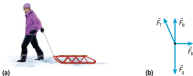
Figure 4 (a) A system diagram of a person pulling a sled. (b) An FBD shows the forces acting on the sled.
