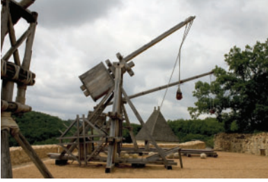
Figure 1 A trebuchet converts the force of gravity downward on the counterweight into the motion of the projectile.
