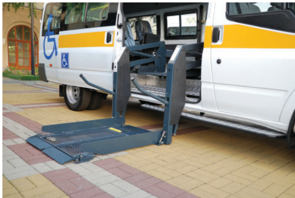
Figure 2 Hydraulic actuators are used in lifts like the one shown here. Hydraulic actuators can exert large forces to lift heavy objects.
